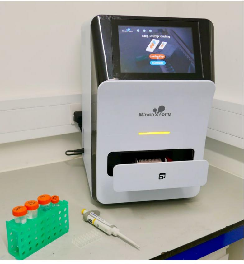
MiNano-form: a high-throughput nanoparticle formulation system and the microfluidic cartridge developed at UCD.
